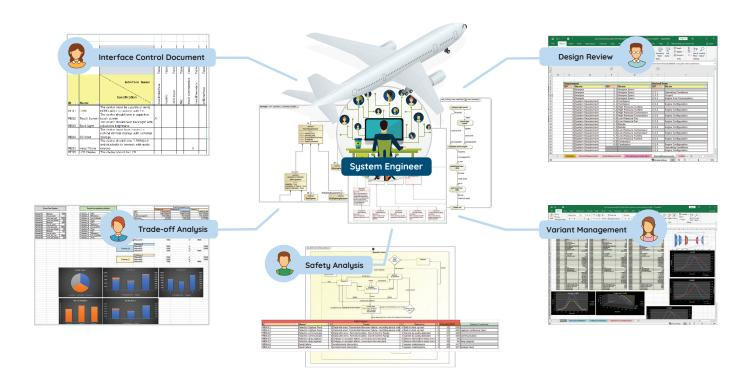
An example of collaboration within an MBSE framework. By using tools such as MapleMBSE, different stakeholders can use simplified, task-specific interfaces to contribute to the overall systems model.
